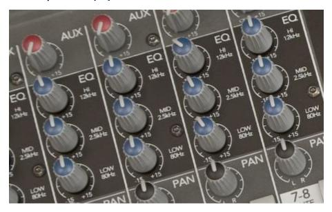
An equalizer is a sophisticated tone control in your mixer or recording software. It's something like the bass and treble controls in a stereo system. Equalization (EQ) lets you improve on reality: add crispness to dull cymbals or add bite to a wimpy electric guitar. EQ also can make a track sound more natural; for instance, it can remove tubbiness from a close-miked vocal.
