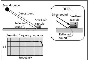
Figure 3. Small mic capsule on the stage floor prevents phase interference.
