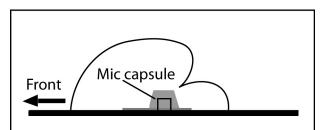
Figure 2. Polar pattern of a half-supercardioid boundary mic (side view)
