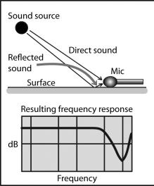
Figure 2. Conventional mic on the stage floor has phase interference at high frequencies.
