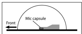
Figure 4. Polar pattern of a half-omni boundary mic (side view)
