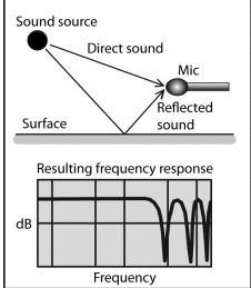
Figure 1. Conventional microphone on a desk stand picks up phase interference.
