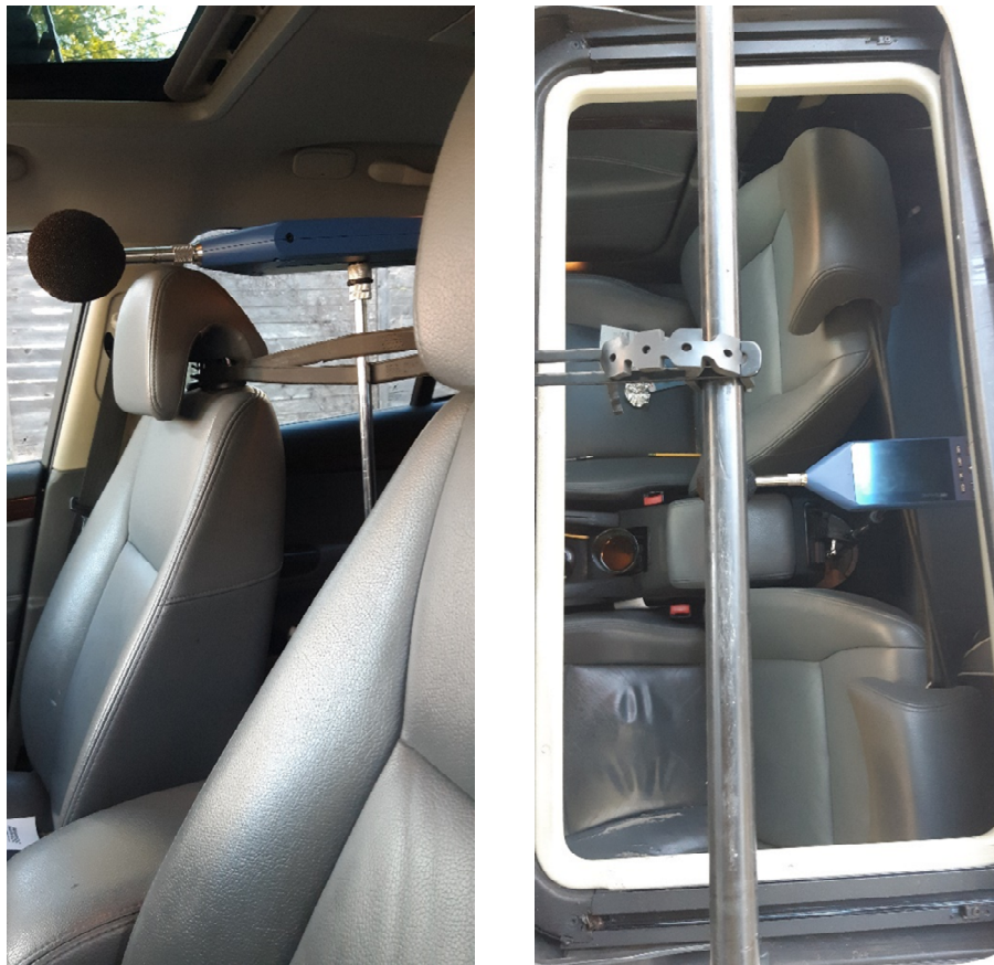
Figure 2 – Position of the sound level meter within the vehicle cabin shown from the side (left) and the top (right)
