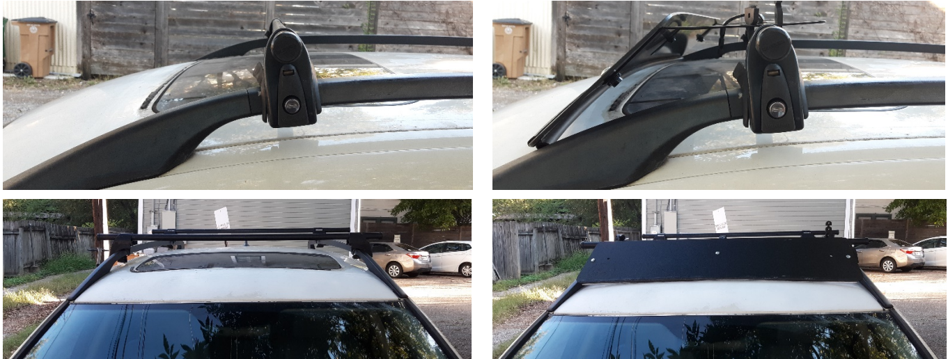
Figure 1 – The vehicle used for this study shown from the driver's side (top) and from the vehicle front (bottom), without the fairing installed (left) and with the fairing installed (right)
