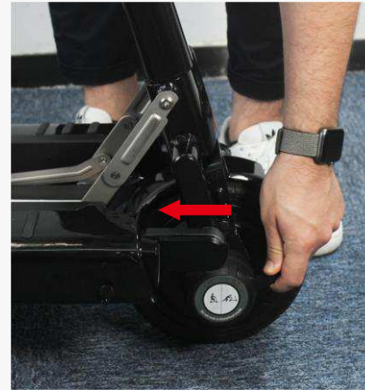
Figure 21. Securing the Freewheel
