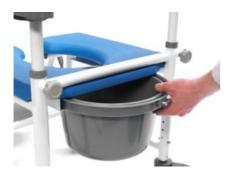
The potty is installed and removed by sliding the potty in to the two rails mounted to the underneath of the seat. To install, slide the potty underneath the seat from the rear of the chair, ensuring the potty sits on both rails of the seat. Ensure nobody is sat on the chair when installing or removing the potty to prevent any trapping risk.
