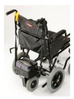
This wheelchair is suitable for some retrofit powerpacks, such as the PowerStroll. A suggested configuration is shown left.
