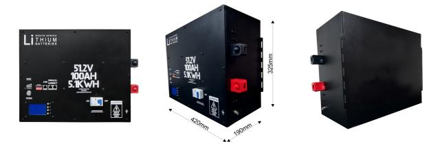
LBSA lithium iron phosphate battery pack is a household renewable energy storage solution developed and produced by Lithium Batteries SA. After fully installation, it is a low-voltage DC battery system with an operating voltage of 51.2V, and works with a low voltage inverter to realize the goal of energy storage for home application.
