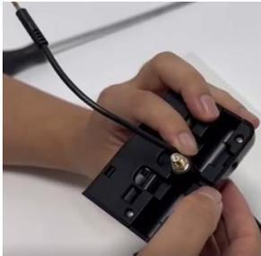
(2) The power cable extends from the back of the camera. You can either thread it through a hole into the vehicle or trim at the reserved port to extend outside the vehicle.
