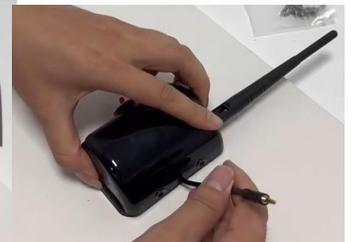
(3) Choose the desired direction for the antenna based on your installation needs. Trim the reserved port for the antenna and install it in the chosen direction.
