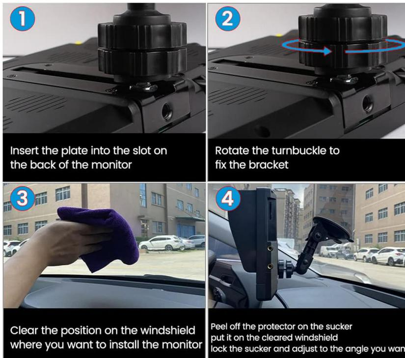
1. Clean and dry the mounting surface where the monitor can be easily seen inside the car, and does not obstruct your vision when driving.
