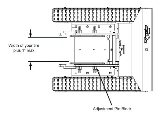
3. Align each tire guide spacer to the nearest hole in the adjustment pin block. Insert the adjustment pin in the nearest hole position to secure in place. Adjusting the spacers correctly will prevent the tire from turning inside the cradle.
