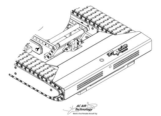
7. Release the latch using the remote controller and move the tug out from under the plane. Drive the tug back under the tire to check that the wheel cradle is set up correctly and to ensure the cradle is latching securely. *When releasing the wheel cradle, the tire should be against the back gate (or cradle adjuster). If not, the latch may not release properly.*
