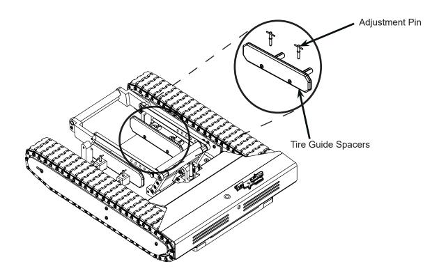
1. If the tire guide spacers are in the widest position and your tire does not fit or it is too close of a fit remove the tire guide spacers and adjustment pins.
