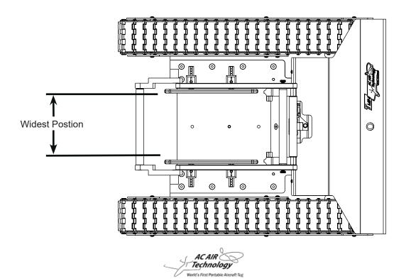
2. Adjust the tire guide spacers by removing the adjustment pin and sliding the spacers towards each other. Ideally the tire guide spacers should be moved the same distance on each side to keep your tire centered in the cradle. The distance between the tire guide spacers should equal the width of your tire plus one inch maximum.
