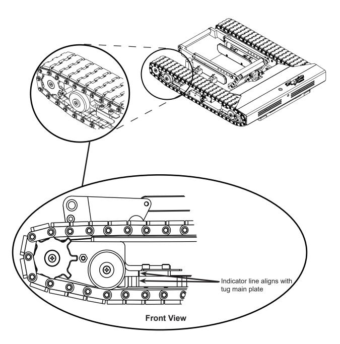
2B-2. Remove 3 cover screws and remove the inside track cover.
