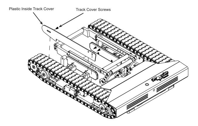
2B-3. Loosen 4 front end retainer screws with an allen wrench and push the front end of the the track to relieve track tension. Temporarily re-tighten the front end retainer screws in the retracted state.
