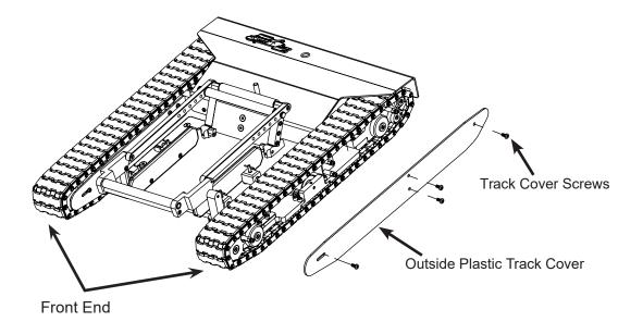
2. Loosen 4 front end retainer screws with an allen wrench. Insert a flathead screw driver into the access slot and push the screw driver towards the tug to leverage the front end of the rail, tightening the track. While holding the screw driver in the desired position tighten the front end retainer screws. IF THE FRONT END OF THE RAIL IS FULLY EXTENDED AND THE TRACKS ARE LOOSE SEE STEPS 2B BELOW. If track tension is successful move on to step 3.
