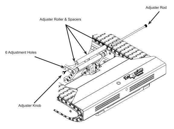
6. Move the cradle adjuster to an adjustment hole near the tire, taking up the space inside the cradle. You do not want the tire to be too tight in the cradle.Leave space between the tire and the cradle adjuster for tire size variations.
