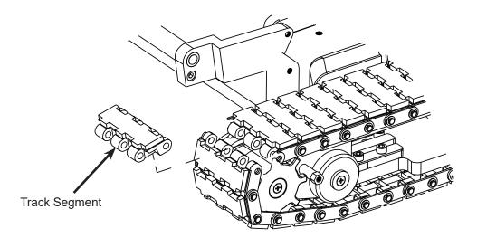
2B-6. Overlap the Track Links on each side of the track and insert the track pin and rotoclip as shown below.
