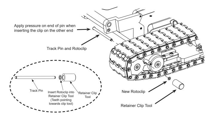
2B-7. Inspect the track pin and Rototclips. The Rotoclips should rotate freely inside the pin groove. Reinstall the Inside Plastic Track Cover. Section 2B is complete, proceed to step 2 for adjusting track tension.
