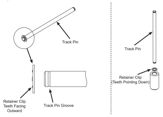
When the retainer clip is properly installed into the track pin groove is should rotate freely inside of the groove.
