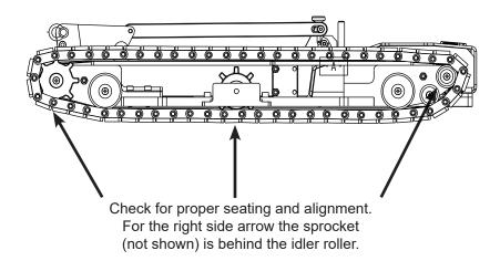
7. Visually check tracks for wear on the treads and wear on the inner plastic surfaces. Also inspect for damaged or missing retainer clips as a result of driving over small rocks. Damaged treads should be replaced before operating the tug.
