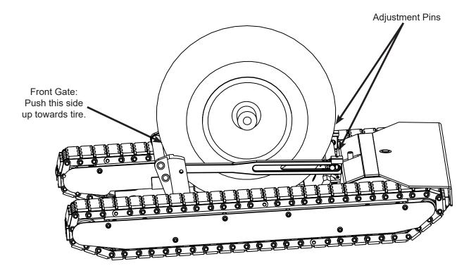
5. Release the latch using the radio and back the tug out from under the plane. Drive the tug back under the tire to check that the wheel cradle is set up correctly and to ensure the cradle is latching securely. When releasing the latch always make sure the wheel is against the back gate. If not, the latch may not release properly.
