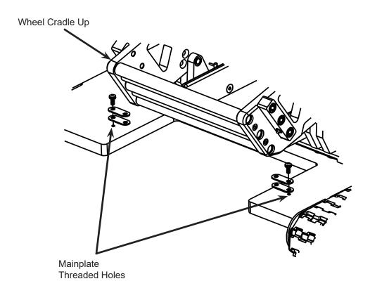
3. Both left and right side shims should be engaged if in the ON position or both sides should be disengaged if in the OFF position to prevent the cradle from twisting.
