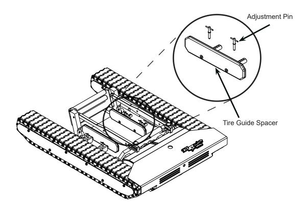
1. If the tire guide spacers are in the widest position and your tire does not fit or it is too close of a fit remove the tire guide spacers and adjustment pins.
