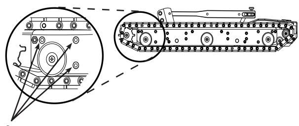
3 Retainer Screws on Outer Side of Rail
