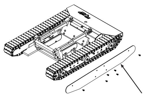
Install Plastic Track Cover Using 6 Screws.
