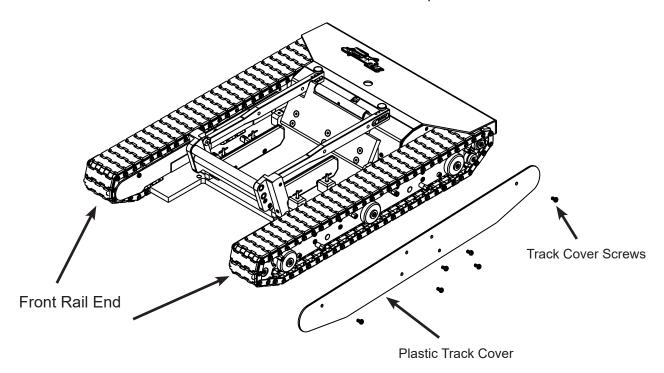
2. Loosen the three front rail end retainer screws. It may be necessary to rotate the large sprocket in order to gain access to one of the retainer screws.
