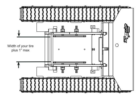
3. Align each tire guide spacer to the nearest hole in the adjustment pin block. Insert the adjustment pin in the nearest hole position to secure in place. Adjusting the spacers correctly will prevent the tire from turning inside the cradle.
