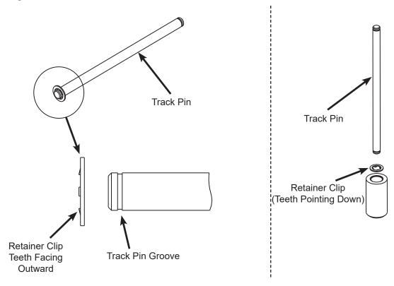
When the retainer clip is properly installed into the track pin groove is should rotate freely inside of the groove.
