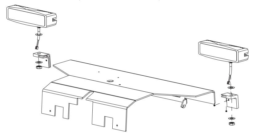
Step 2. Route the light wires as shown if the picture below. Note: wires need to be tucked up close to clear the tracks.
