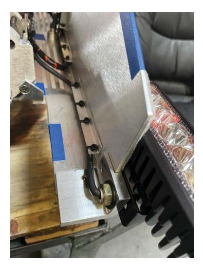
Step 3. Zip tie the wires as shown below. The green arrows are for new zip ties. The red arrows are existing zip ties that need to be reinstalled.
