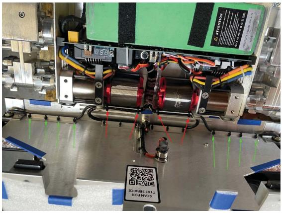
Step 4. Run wires through the wire manager shown below with the red arrow. Connect plugs to PC board shown with green arrow. Note: Green arrow connections are interchangable for right and left light wires.
