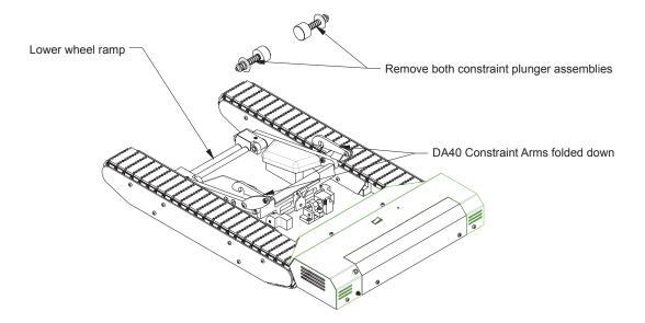
2. Load the front wheel of the plane onto the tug with the wheel ramp in the full up position.
