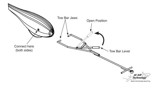
10. Close the tow bar jaws to secure the tow bar into the front wheel.
