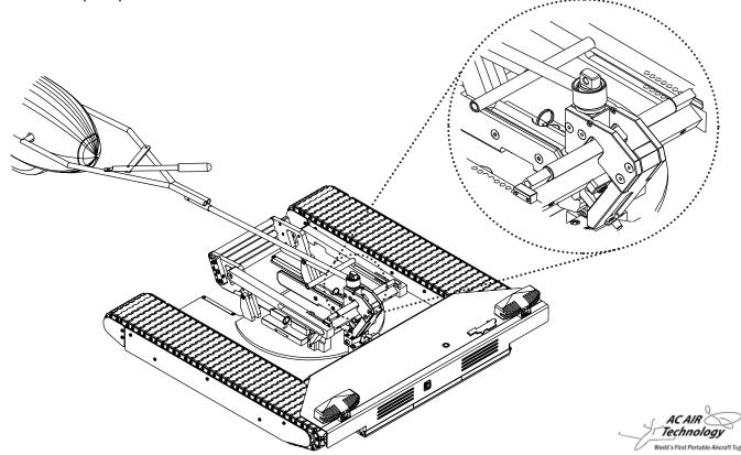
3. Reinstall the post cap and pin to secure the tow bar onto the adapter.
