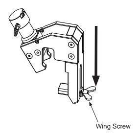
4. Postion the wheel cradle in the up-position and confirm that the cradle latch is fully engaged. Position the adapter over the lazy susan back gate.
