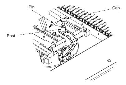
2. Maneuver the tug over to the tow bar and position the tow bar connecting ring onto the adapter post.
