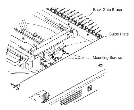
Note: The guide plate and mouting screws are installed once. They will not need to be removed for normal, non-cirrus, tug use.
