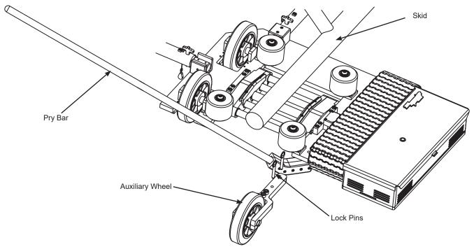
3. Slide the auxiliary wheel onto the tug main plate and align the pin holes with the holes on the main plate. Insert the 2 pins into the holes to lock the auxiliary wheel in place.
