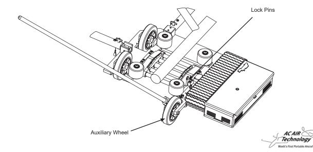
3. Repeat steps 1-3 for the second auxiliary wheel. Position the pry bar as shown below.
