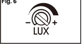
The LUX control knob can be adjusted for the surrounding level of darkness needed to activate the motion sensor (Fig. 6). This is quite variable. The far left position (-) sets for maximum level of darkness. The far right position (+) sets for a minimum level of darkness.
