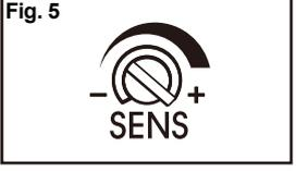
The SENS control knob can be adjusted to control the range of the motion sensor (Fig. 5). The far left position (-) sets the motion sensor range to approximately 0.3m. The far right (+) sets the motion sensor range to approximately 9m.
