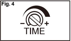
The TIME control knob can be adjusted to control the length of time the light stays ON when triggered by the motion sensor (Fig. 4). In the far left position (-), the duration time is approximately 10 seconds. In the far right position (+) the duration time is approximately 30 seconds.
