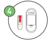
Remove one side of the liners and stick each pair of strips as shown. Press firmly.
