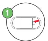
Remove cover by pushing catch in and up.
