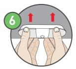
Allow space on either side for removal. Press the light firmly to the surface for 30 secs.
