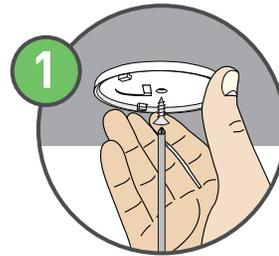
Mark the centre mounting hole in the cover and drive the screw into the mounting surface.
