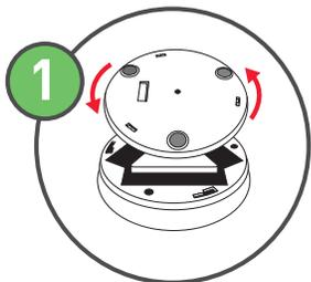
Remove the cover by rotating counter-clockwise. Ensure surface is clean from dust and grease (do not use household cleaners).
