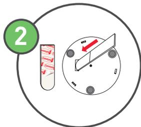
Remove the red liner and insert the tab into the slot. Press the strip onto the back of the cover.
