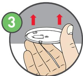
Remove the black liner of the adhesive strip and then press and hold the base onto the surface for 30 seconds.
