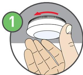
Turn counter-clockwise to release the light from the cover.
