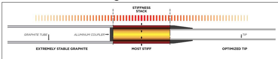
*This Stiffness Stack™ is 2.5x stiffer than a traditional wedge shaft and allows the kickpoint to be optimized for the perfect launch and trajectory.*
