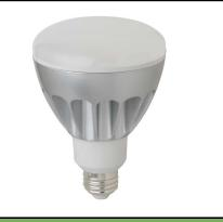
The ETi 12 watt 800 lumen BR30 LED lamp offers exceptional performance for precision lighting applications, while reducing energy and maintenance cost when compared with conventional light sources. They are UL listed for use in damp & dry locations and are RoHS compliant with no lead or mercury. Warranty is 5 years or 60 months.
