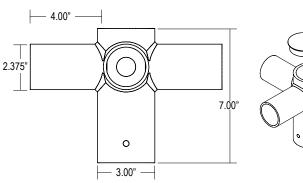
**TH490** shown. All tenon configurations conform to the same tubing and tenon dimensions.
