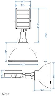
Reflector Dimensions shown. Reflectors sold separately. Type 5 19" (SLR-9): 19" OD x 12" H
