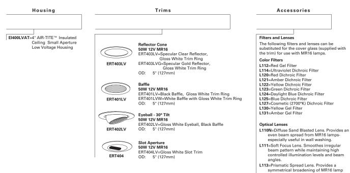
symmetrical broadening of MR16 lamp beams. L115=Fans the MR16 beam to produce a
