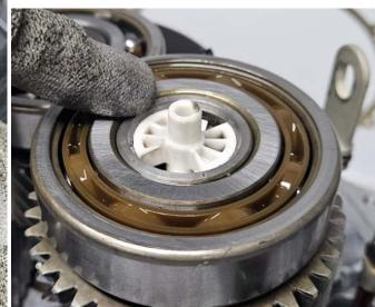
Before reassembly, ensure all bearings are flushed with brake cleaner, lightly lubricated with drive unit oil and run smoothly. Failure to do this could cause irreversible damage to the motor internally and cause noisy operation.
