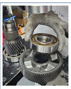
• When fitting the new intermediate shaft gear, ensure that the proud face is facing the bearing. As indicated in the beside picture.
