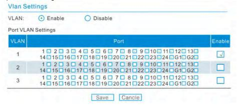
Check box is used to divide the port VLAN and enable VLAN, click "Save" to save settings and enable port VLAN function.
