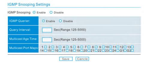
IGMP snooping can work with GMRP, when device of network change connection port. Send GMRP notice to prevent multi-cast information from missing. Query Packet for IGMP is used to query existing multi-cast group, Query interval is according to Query Interval in web page above .If MAC address have not refreshed within aging time, switches will delete multi-cast group, and not send leaving message when deleting.
