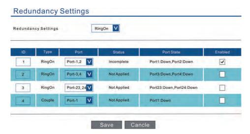
Redundancy Settings: can select RingOn after setting, save setting parameters, then RingOn will be enabled. To set RingOn function and related parameters, please refer to the following forms.
