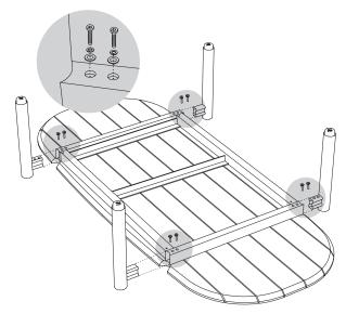
2 Stand upright and adjust leveling feet as needed.
