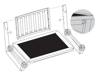
3 Secure base to legs with six 40mm Bolts.
