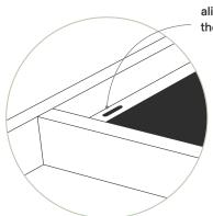
Backrest slots should align with the back of the armrest, as shown
