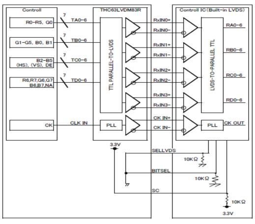
$\ensuremath{\texttt{SELLVDS}}$  signal line has 10 k  $\Omega$   $\ensuremath{\,\text{pulldown}}$  resister
