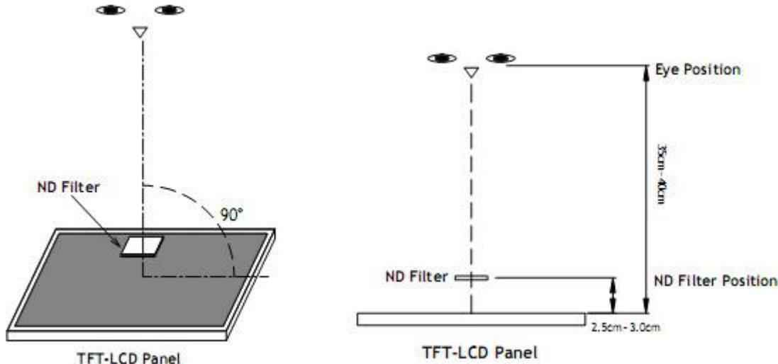
**Bright dot:** The bright dot size defect at black display pattern. It can be recognized by 2% transparency of filter when the distance between eyes and panel is  $350\text{mm} \pm 50\text{mm}$ .
