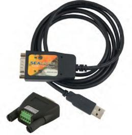
The USB serial adapter features programmable baud rate and data formats with 128-byte transmit and 384-byte receive buffers. The adapter is compatible with all standard PC baud rates and supports high-speed communication to 921.6K bps. The 2107 is powered by the USB port and status LEDs molded into the enclosure indicate serial data activity and connection to the host.
