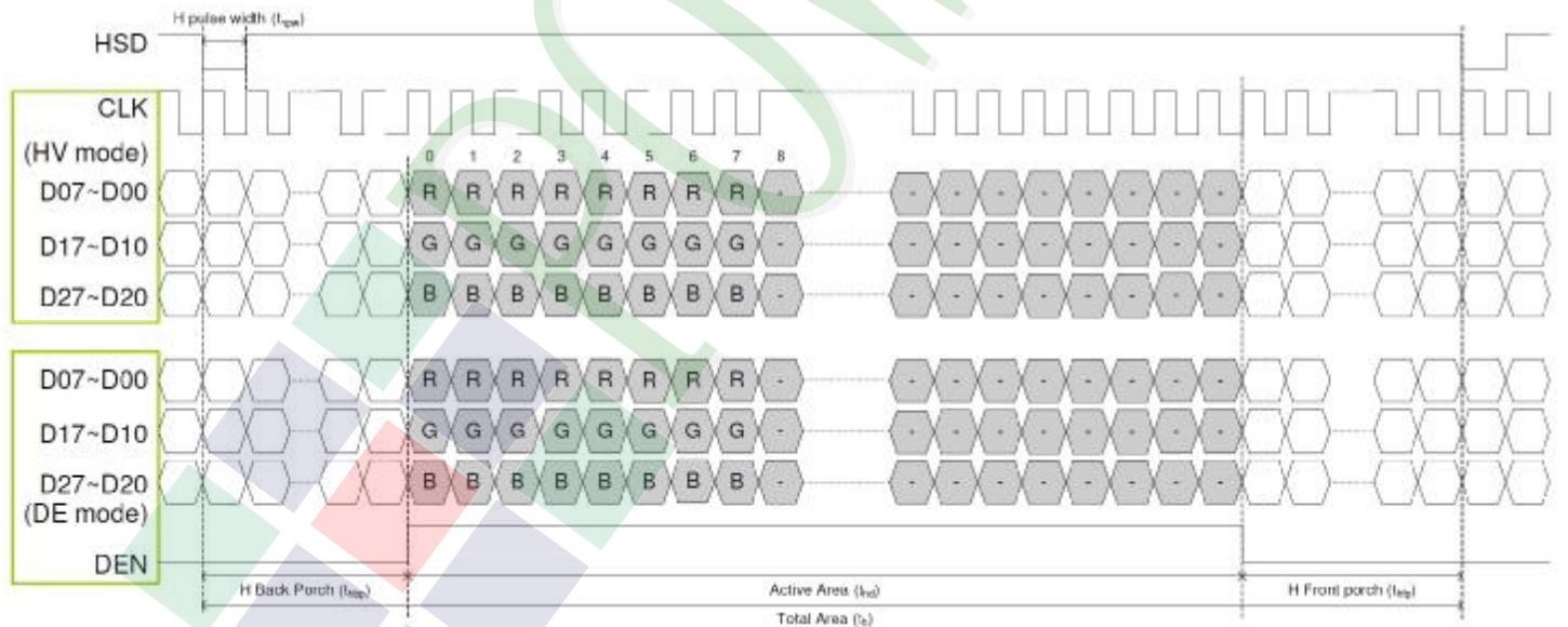
Horizontal input timing diagram
