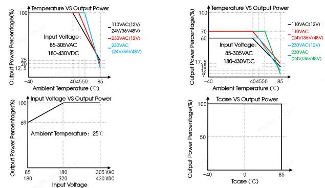
Note: 1. With an AC input voltage between 85-180VAC/180-320VDC, the output power must be derated as per the temperature derating curves; 2. This product is suitable for applications using natural air cooling; for applications in closed environment please consult Mornsun FAE.
