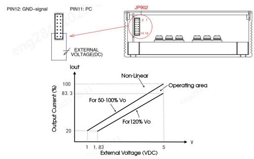
\*Note 1: By factory default, the output current adjustment function is not activated, and the Vccs (Pin13) and PC-DIS (Pin14) are shorted. When this function is not required, short-circuit the Vccs (Pin13) and PC-DIS (Pin14). Otherwise, the power supply has no output
