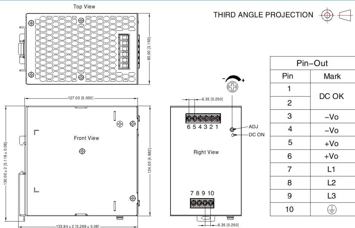
10, 11 any position must be connected to the earth(
