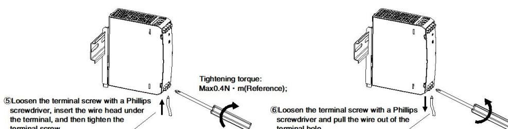
Note: Keep the following installation clearances: 20mm on top, 20mm on the bottom, 5mm on the left and right sides are recommended when the device is loaded permanently with more than 50% of the rated power. Increase this clearance to 15mm in case the adjacent device is a heat source (e.g. another power supply).
