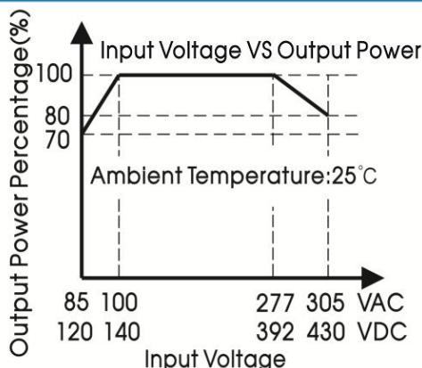
Note: 1. With an AC input voltage between 85 - 100VAC/277 - 305VAC and a DC input between 120 - 140VDC/392 - 430VDC the output power must be derated as per the temperature derating curves;
