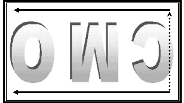
RPF = high: display with 180degree rotation
