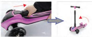
On the bottom of the handlebar stem is a lock which keeps it in place. Twist it so that it is in the "open" position, and then pull it towards the rear wheel of your scooter.
