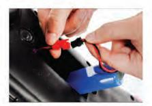
2. Once the battery compartment is open, plug the charging cable that is connected to the battery into the cable in the battery compartment. Close the battery compartment and screw the cover back on.
