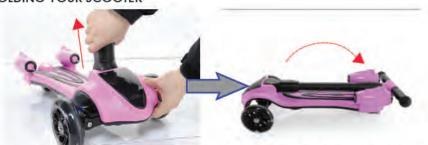
On the bottom of the handlebar stem is a lock which keeps it in place. Twist it so that it is in the "open" position, and then pull it upwards.
