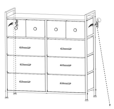
a:First, according to the size of the accessory  $\bigcirc$ , draw the position that needs to be punched on the wall. Punch holes in the wall according to the mark position.
