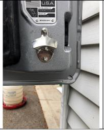
Using the Bottle opener as a guide, position it on the swing gate as shown. (note the top of the bottle opener is about ¼" down from the lip for the JL Badge). Use a Marker to mark the center of your top hole.
