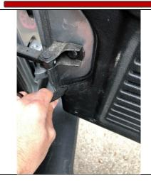
First Step will be to remove the black panel from the Swing Gate. Give a light tug on the fabric cable loom so it applies a little pressure to the panel. This will either pop off the first clip, or make a gap large enough for you to grab the perimeter of the panel. Work your way around the outside of the panel pulling straight out as you go in order to remove the swing gate panel.
