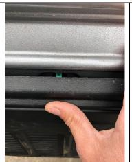
Line up the clips of the black panel with the corresponding openings in the swing gate.
