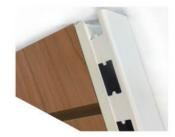
The panel is now ready to hook into the columns. This is a 2 person task. For wall bays get the the panel standing against the wall with columns close by. Tilt the panel sideways on one corner and bring the column and panel together as shown. When one side is fitted and hooks have fully dropped into the column do the other edge. Panel and columns should then be plumb.
