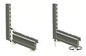
Using a mallet tap the baseleg until the lug can go no further in the H slot. Unwind the adjustable foot disc a few turns in preparation for levelling later.
