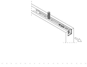
E: Simultaneously slide and pivot the leading edge of the door out of the system to reveal the rear hanging bracket.
