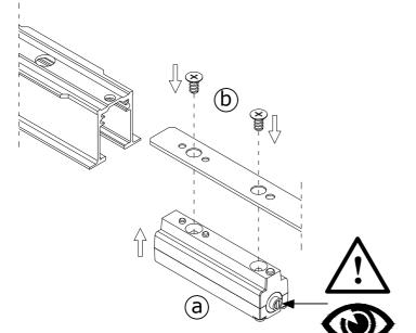
Slide the Touch Latch and stop-bar back into the track in the same orientation it was removed.
