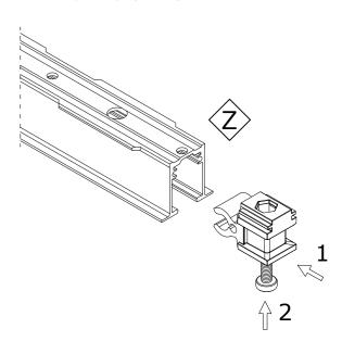
(a) Insert the track back into the pocket door system in the reverse order of removal.
