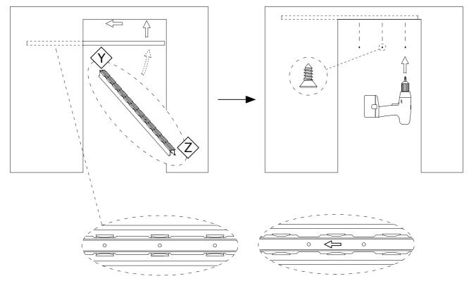
Remove the rear hanging bolt from the original rear hanging bracket and insert it into the replacement rear hanging bracket provided in the Touch Latch box.
