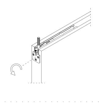
F: Remove the 3 screws holding the rear hanging bracket into place and slide this free of the door.
