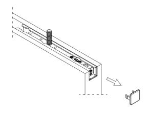
C: Insert black grub screws into the lower hole in the leading hanging bracket (this lifts the locking lever).
