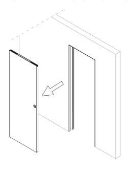
B: Remove the grey cap off the leading edge of the door at the top to reveal the brackets.
