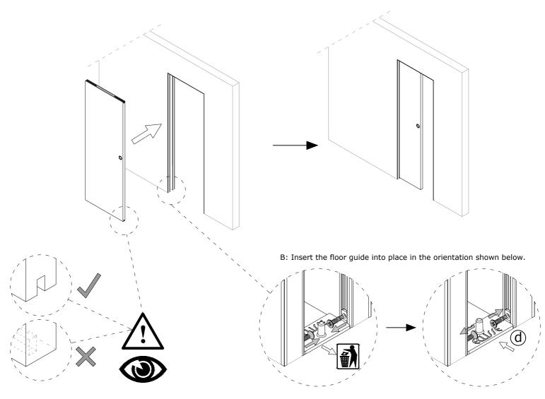
C: Slide the new rear hanging bracket into the back of the door and secure in place with 3 screws. Slot the door back into the pocket half way and insert the leading hanging bracket. Once in place, remove the black grub screw from the lower hole and screw it back in the upper hole to lock the bracket into the door.
