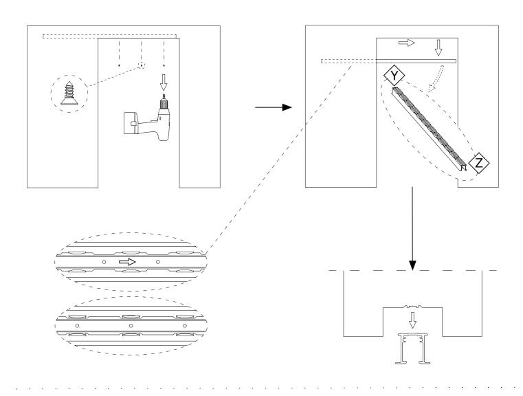
(3) Remove the leading adjustable stop from the track and remove the runners.
