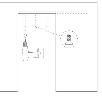
Remove track from the pocket unit by removing the small screws holding the track to the header across the opening. Slide the track to one side and it will drop out. NOTE: Please store these screws safely
