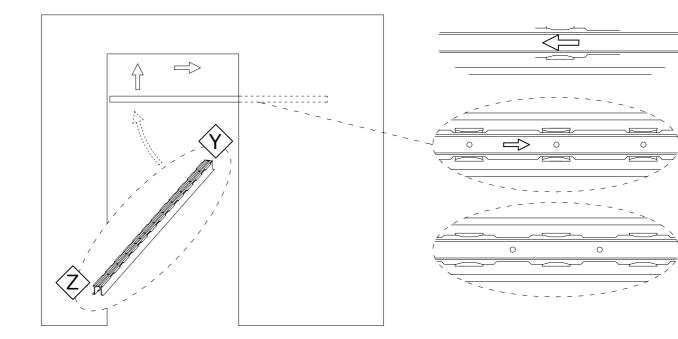
Insert the track back into the pocket system in reverse order of removal
