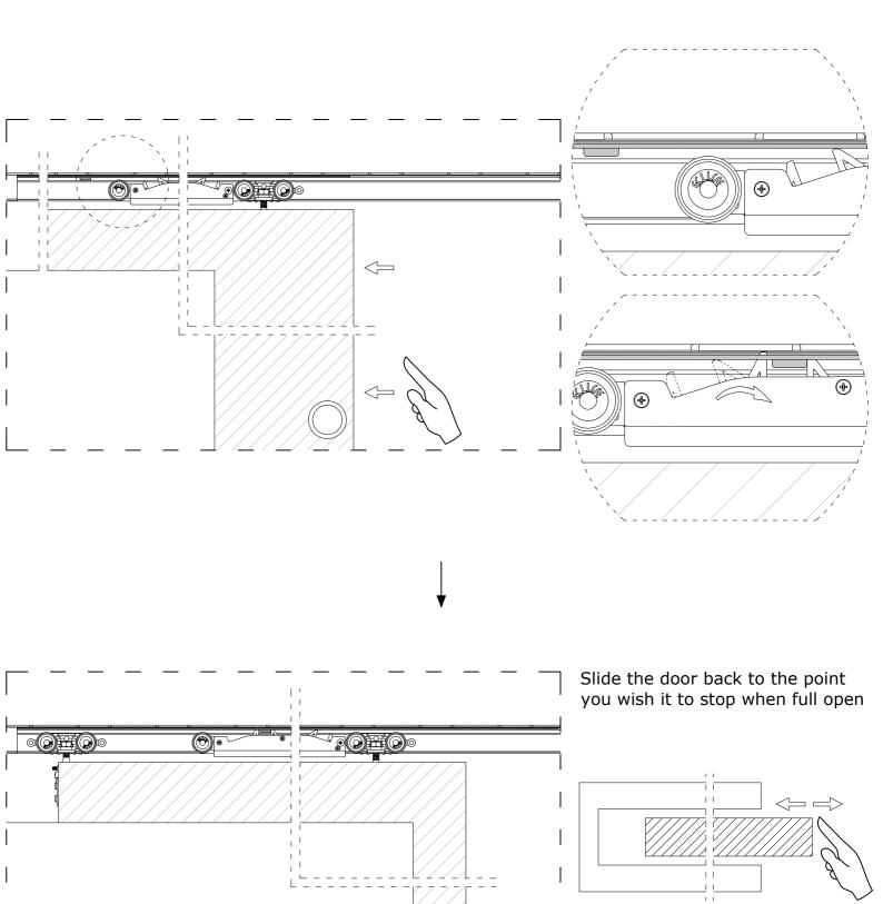
With the door open to your desired position, pre-drill and screw the bar to the top track to fix into place
