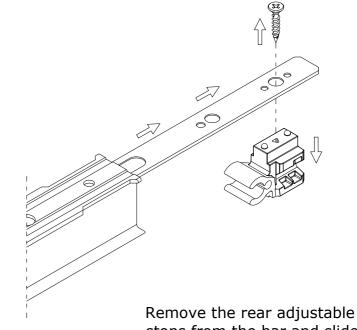
stops from the bar and slide the bar back into the track
