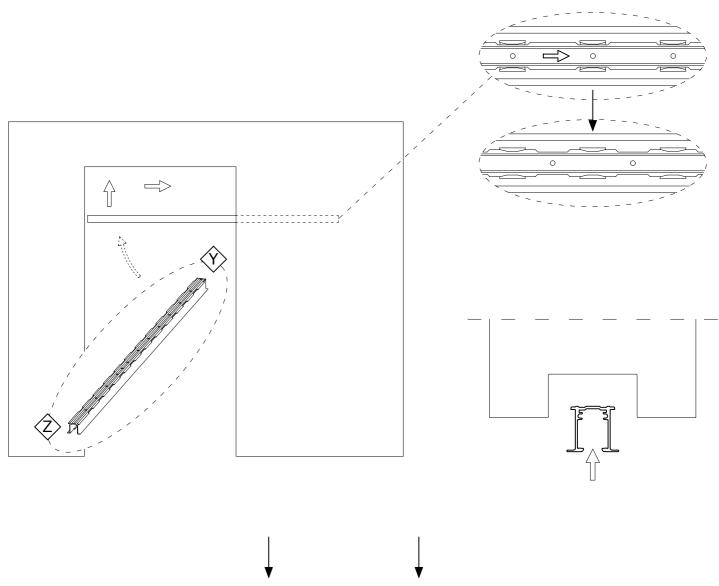
Insert the track back into the pocket system in reverse order of removal
