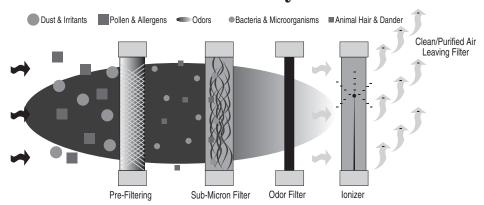
The above is an illustration of how the  $HEPAtech^{TM}$  air purification systems work. Dust and other irritants are pulled into the air purification system and cleaned through the  $HEPAtech^{TM}$  Filter. Clean, purified air is released into the room.
