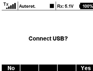
After some seconds, a window with the internal memory of Jeti transmitter open on your PC. Copy the "BRAIN.bin" file in to the "Devices" folder of your Jeti transmitter and after this close the Window and push the "Esc" button in your transmitter;
