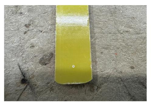
f. Drill and tap the hole and put the G10 plate back in and secure the stab and now do the same on the other side.
