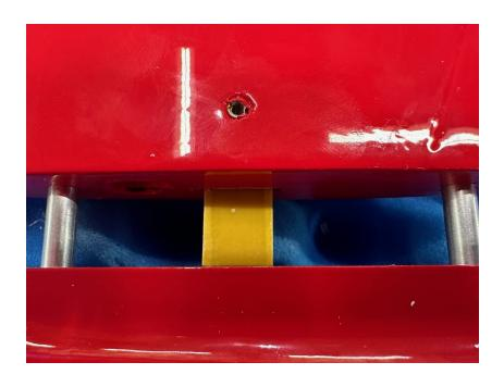
e. Drill on the mark with a 2.5mm drill bit and then tap the hole with your 3mm tap and test fit. The tip can be removed at this point and installed later for good. We will talk about how to install the tip light later.
