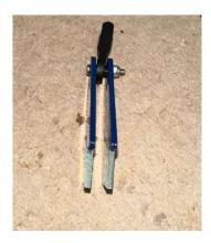
c. Slide the control horn into the surface and outline with low tack masking tape.
