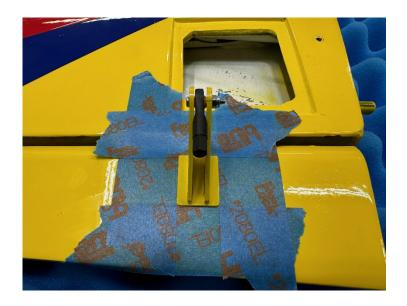
d. Remove the control horn and scuff the portion that will get epoxied/hysoled into the surface as well as scuff the section under the base plate.
