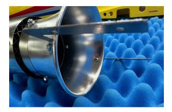
b. Slide the tube in and then mount the second tab.
