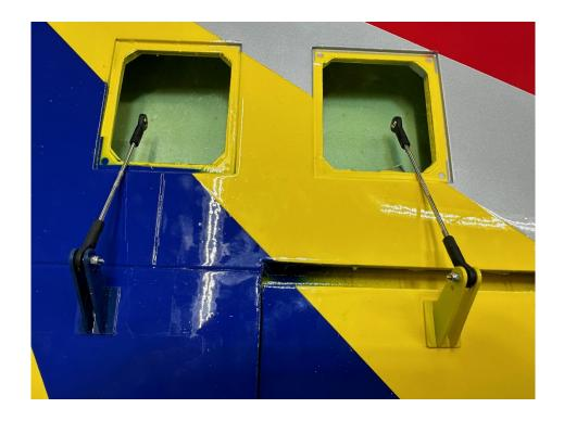
b. Aileron pushrods will be about 112mm and the Flap pushrods will be about 105mm.
