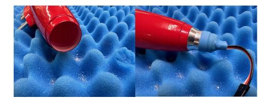
a. Once the light fits snuggly into the tip tank, connect the extension and run it out the tank and the back hole that will match up to the hole on the wing. Then epoxy/ Hysol in the light and let dry.
