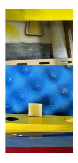
c. Scuff up the top and bottom of the G10 plate that will be epoxied into the wing. Then glue them into the wing. Slide the wing back onto the tubes
