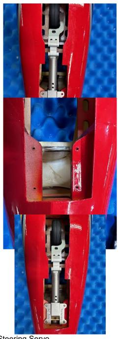
10. Installing the Nose Wheel Steering Servo
