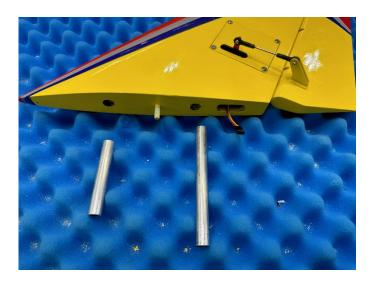
b. Hysol/ epoxy the tubes into the fin and let dry.
