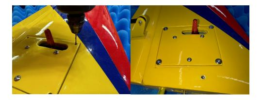
e. The push rod to be used here is the 40mm one, thread on two ball links to about 72mm and power on the servo and test fit the pushrod and adjust to the proper length.
