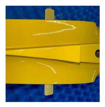
c. Test fit the stab to make sure everything lines up and the stab fits flush against the fuselage.
