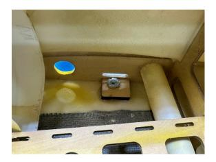
f. Slide the wing into place and hold it tight against the fuselage, use a 4mm tap and mark the G10 plate. Then drill the mark with a 3.5mm bit. Then tap the G10 plate.
