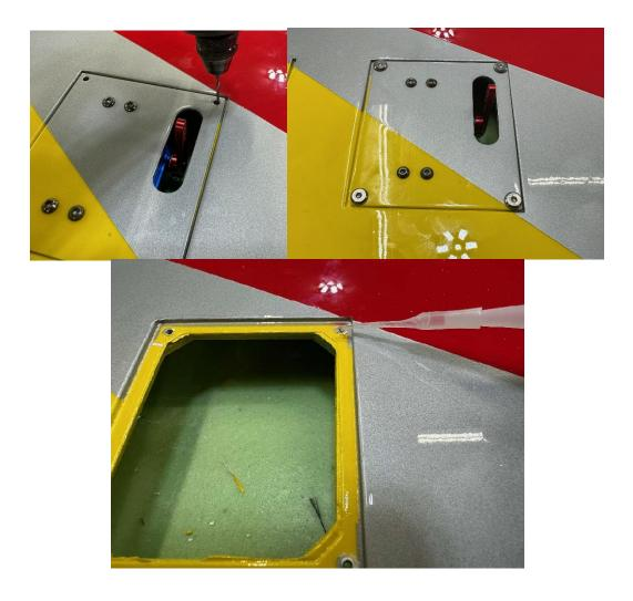
f. Do the same on the other wing and then run and install the servo extensions for the ailerons and flaps.
