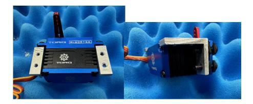
d. Use the 3mm Phillips head screws to secure the servo to the servo hatch,
