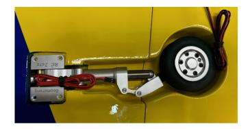
b. Using a 2mm drill bit drill one hole at a time and thread in the counter sunk Phillips head screws. Remove and take the landing gear out and put a drop of thin CA into the hole to harden the thread.
