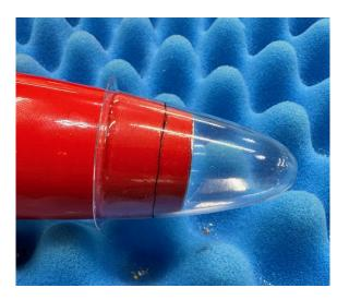
c. Once trimmed to fit, epoxy/ Hysol the lens in place. At this point you are done unless you want to paint like we did. Mask off the area you want to paint and then paint.
