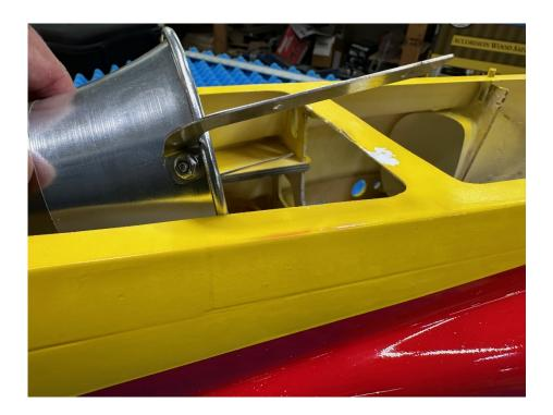
c. Slide the tube into the mounts in the tail and line up the ears at the front end, then screw the tube into position.
