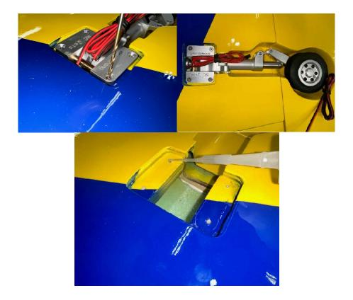
d. Do the same for the other side, then re-install and run all the wires for the gear and brakes.
