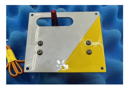
e. Test fit the servo into the bay and drill the holes for the servo hatch screws and tap them. Then put one drop of CA in each hole and let air dry.
