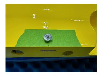
e. Drill the hole for the blind nut with a 5.5 mm drill bit, then insert the blind nut inside the fuselage and pull it into the plywood.
