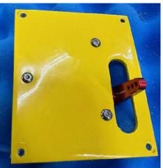
c. Fit the servo into the stab, it might be necessary to trim the lip a little bit depending on the servo you have picked to use.
