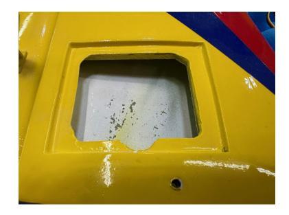
d. Once fit, drill the holes for the servo hatch screws and then tap, and harden the threads using thin CA.
