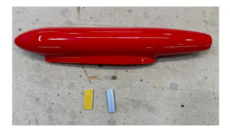
b. Using a 3mm tap clean out the screw hole in the bottom of the wing at the tip.
