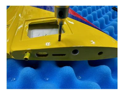
e. Slide the stab onto the tubes and G10 plate and hold in place and mark where to drill the hole, we use a sharpened 3mm bolt to mark the center of the G10 plate. Then remove the G10 plate and drill the hole.
