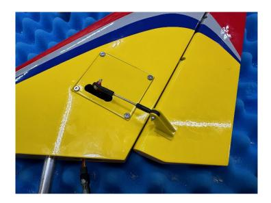
e. It might be necessary to clean the threads on the nylon bolt on the bottom of the fin, to do so use the wing nut that will hold the fin on later on, gently thread a little and then back it off and work it slowly till all the threads are clean and the wing nut goes on easily.
