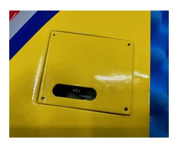
e. Drill and tap for the screws to hold the hatch on, then remove the hatch.
