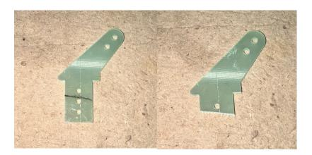
3. Once trimmed, if you want to paint the control horns and flat plates this is the time to do it. We take an empty cardboard box and put slices in for the control horns and then lay down some double-sided tape to secure the flat plates.
