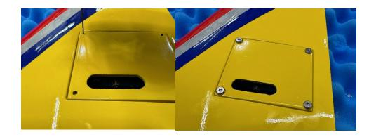
f. Remove the hatch and put a drop of CA into each hole to harden the threads.
