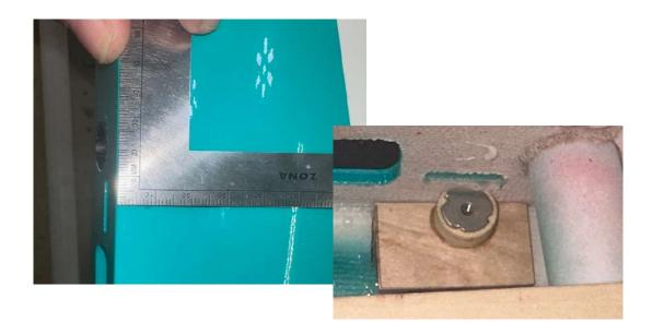
20. Then taking an extra 3mm bolt and putting a point on it we will use this to make a mark on the fiber glass tab in the wing to show where to drill your mounting hole.
