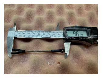
11. Install the pushrods and secure the hatch.
