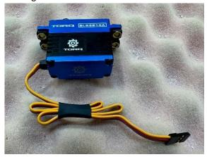
5. Test fit the servo into the hatch and using the 1.2 mm drill bit drill the holes for the servo screws, then tap them with the servo screws and put a drop or two of thin CA in each hole and allow to air dry.
