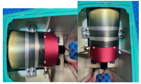
37. Make sure that you have about ¼- ½ inch of the tail pipe on the turbine exit the fuselage. Make sure the turbine is square and go ahead and drill the mounting holes for the turbine and then using thin CA again harden the threads.
