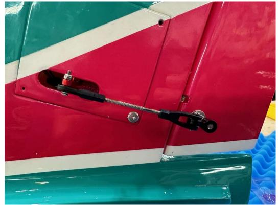
29. Install the nylon end of the control horn on the post, then assemble the pushrod to about 80mm end to end. This will have to be fine tuned to your model but is a good and close starting point.
