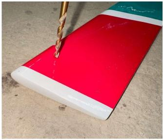
6. Using a 2.5mm driver install the control horn through the rudder and once through put a tiny drop of Loctite on to secure the bolt in place.
