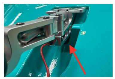
12. It may be necessary to trim a little bit of the fiber glass for the landing gear to drop into position.
