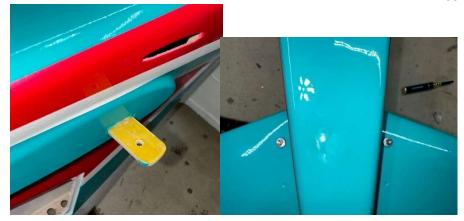
25. Locate the indents in the elevators and drill them out with a 3.5mm bit to allow the control horns to pass through the elevator and install with washer and nut, then thread on the nylon control linkage.
