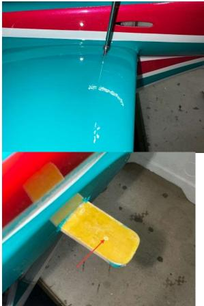
24. Drill on the mark and the test fit the stab and remove.
