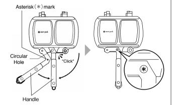
If you feel the handle is loose when you set it, return the handle to the original position, and adjust the fitting as follows.
