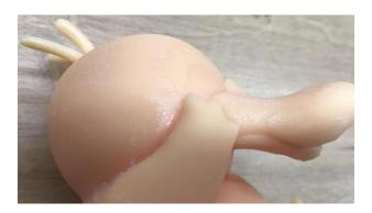
(9) The whole surface exposure layer appears in the printing process: a. Check the slice image of the whole layer in the slice data, and check whether there is any error in the original stl file; b. The LCD printer screen abnormally exposes /DLP light machine exposes: restart the device / contact the after-sales service.
