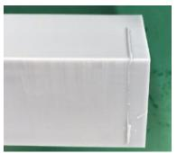
(7) Obvious surface texture: a. Check whether the release film of the liquid tank is tight (aging/deterioration of elasticity); b. Reduce the platform lifting speed (30%) or the other suitable amount.
