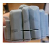
(5) Leakage of liquid tank: Pour the resin in the liquid tank back into the resin bottle after filtering. Check whether there are sharp solid residues at the bottom of the liquid tank/forming platform surface/LCD screen surface, clean and replace the new release film in time.
