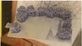
(2) The formed part and the support are disconnected from the support connection: In the slicing software, increasing the depth of the support embedded in the part (0.5mm), increase the support diameter, and the support distance/density appropriately.
